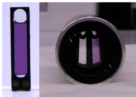
Figure 2. Photographs of the separated, (6,5) rich, length sorted SWCNT population used in this work (1 mm path length), and as diluted for measurement in the sector-shaped AUC cell. The dispersion is richly colored due to the strong intrinsic optical transitions of the SWCNTs, and the high purity of the sample.
